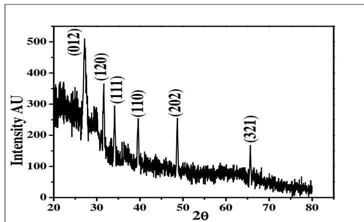
The data matched with that from the JCPDS data card [20] and the planes (012) and (110) correspond to rhombohedral phase. The observed data matched with JCPDS card [21]. This data confirmed the material. The crystallite sizes calculated are systematically tabulated in the table 4.1. The structural parameters of Bi-doped SnO<sub>2</sub> thin film samples are represented in Table 2. Crystalline nature of the films is clearly seen from the data.
